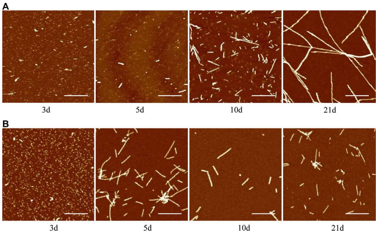
**Fig. 3.** Morphological changes of A $\beta$  with time as monitored by AFM. A $\beta$  alone (A) and A $\beta$  + 10 mM  $\beta$ -CD (B). AFM imaging was carried out in air using TMAFM. Scale bar = 500 nm.
